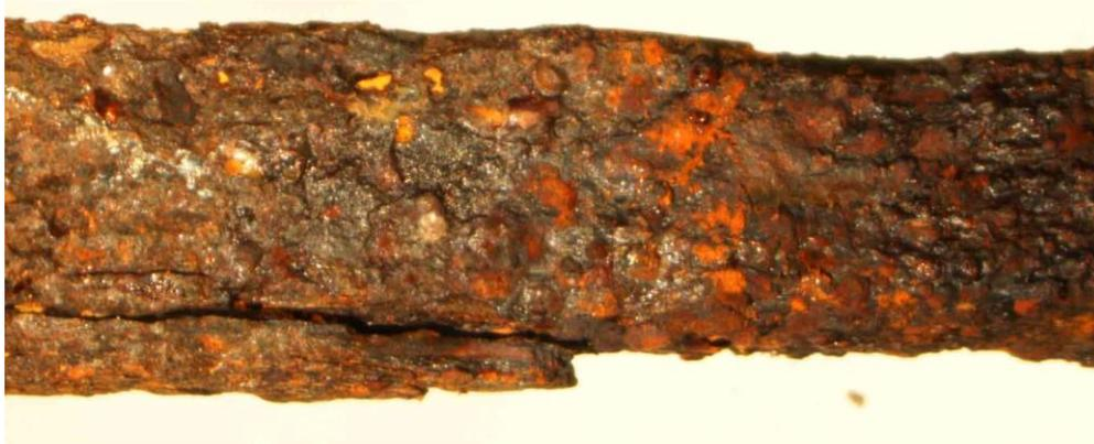
*Figure 8. Nail 0014/6: corrosion pustules and lamination of corrosion product at metal/corrosion layer interface.*
