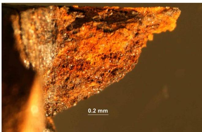
Figure 1 – Sample 0014/: soft powdery corrosion on nail surface.
